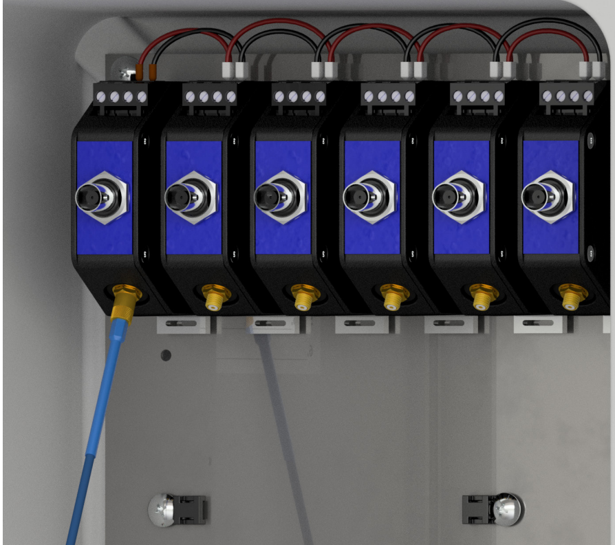
Figure 11. Connecting Proximity Probes
