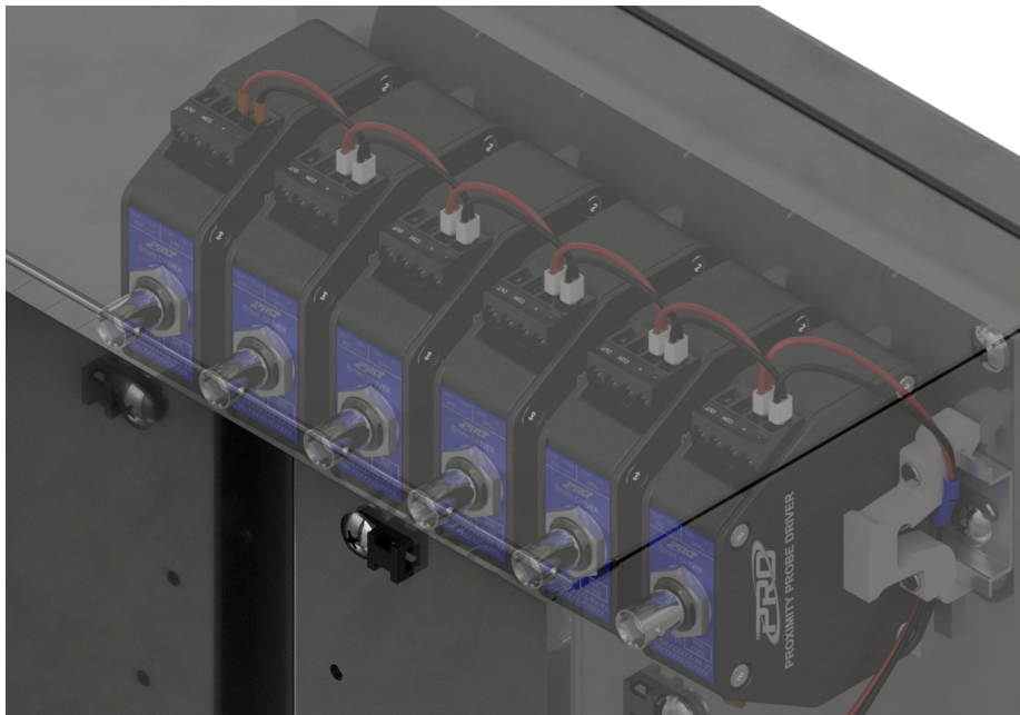
Figure 10. Power Routing for Probe Drivers
