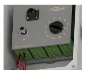
Figure 11. Connecting Cables to Modular Switch Box (SSB1001)
