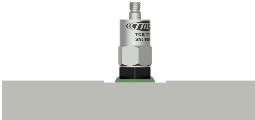
Figure 2. Adhesive Mounted Sensor
