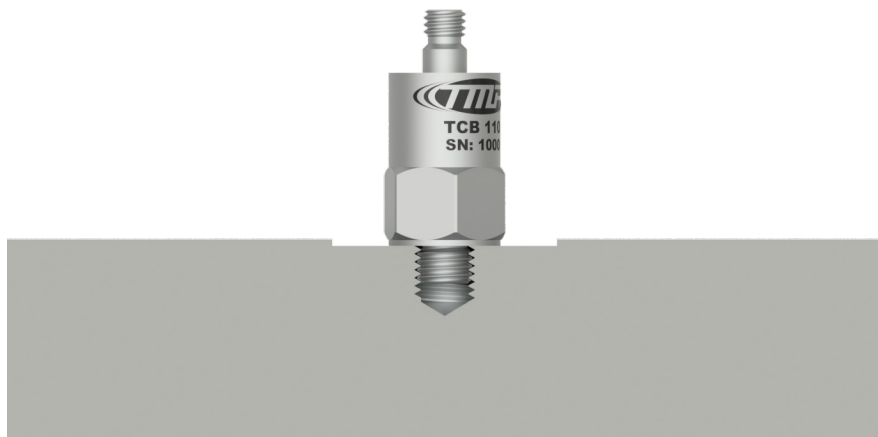
Figure 1. Stud Mounted Sensor
