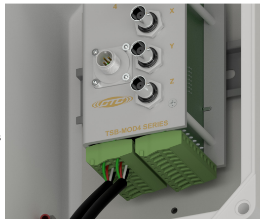
Figure 11. Connecting Cables to Modular Switch Box (TSB1001)
