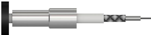
5. Fan out the shielding.
