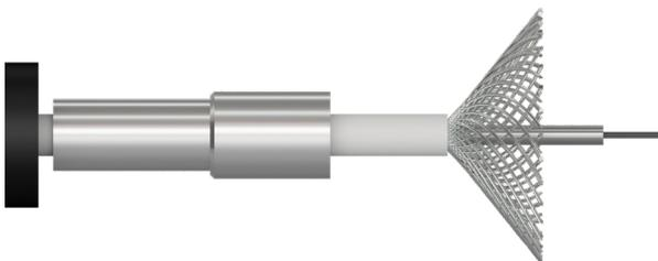
6. Insert conductor into the connector so that the inner conductor rests on the tray.
