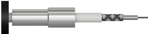
5. Fan out the shielding.
