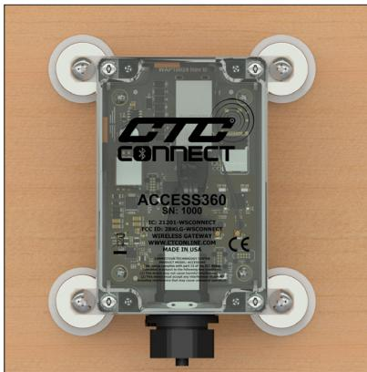
3. Repeat this process for the remaining three screws.
