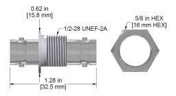
Isolated BNC to BNC Bulk Head Connector, Nickel-plated Brass with NORYL® Insulator
