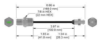
2 Pin MIL (316L Stainless Steel) to BNC Jack (Nickel-Plated Brass), Adapter Cable (Polyurethane) with 0.5 in. (12.7 mm) Pipe Thread Adapter
