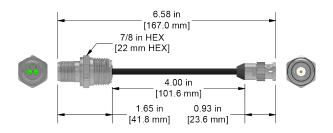
2 Pin MIL (316L Stainless Steel) to BNC Plug (Nickel-Plated Brass), Adapter Cable (Polyurethane) with 0.5 in. (12.7 mm) Pipe Thread Adapter
