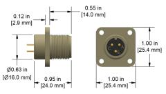
3-Pin Flange Adapter, for use with CTC's 3-Socket MIL-style Connectors, Aluminum
