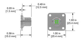
4- Pin Flange Adapter, for use with CTC's 4-Socket mini-MIL Connectors, 316L Stainless Steel
