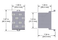
Terminal Block, Four Position, DIN Rail Mountable, for use with SCE Junction Boxes
