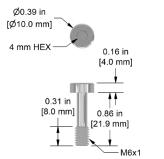
M6x1 Captive Bolt with Socket Head Cap for TREA/TRCA Series Compact Triaxial Accelerometers, 18-8 Stainless Steel, 0.89 in. (22.6 mm) Length
