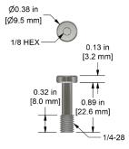
1/4-28 Captive Bolt with Socket Head Cap for TREA/TRCA Series Compact Triaxial Accelerometers, 18-8 Stainless Steel, 0.89 in. (22.6 mm) Length
