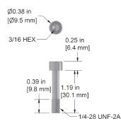
1/4-28 Captive Bolt with Socket Head Cap for TXEA/TXFA Series Large Triaxial Sensors, 18-8 Stainless Steel, 1.19 in. (30.23 mm) Length
