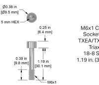
M6x1 Captive Bolt with Socket Head Cap for TXEA/TXFA Series Large Triaxial Sensors, 18-8 Stainless Steel, 1.19 in. (30.23 mm) Length
