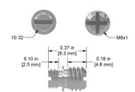
10-32 to M6x1 Adapter Stud, 303 Stainless Steel, 0.37 in. (9 mm) Length
