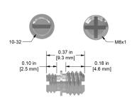
10-32 to M5 Adapter Stud, 303 Stainless Steel, 0.31 in. (8 mm) Length
