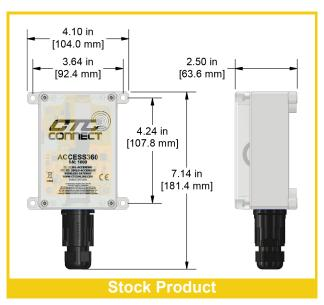
\*The ethernet cable backshell for ACCESS360 is built to accomodate an industry standard RJ45 Ethernet connector.
