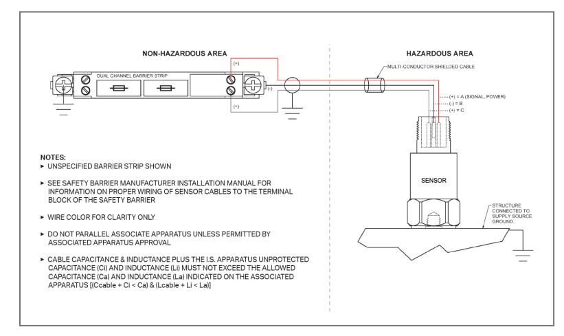
This is an example of a control drawing for a vibration sensor.
