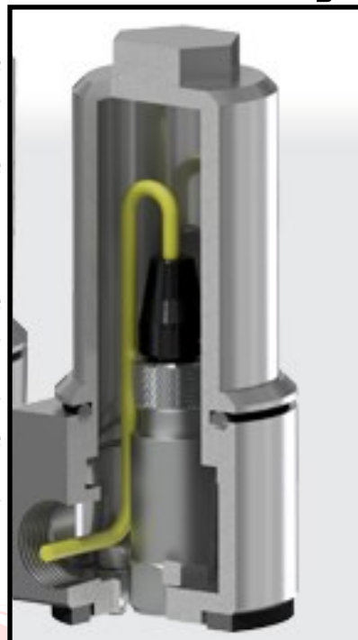
Fig. 2. Cutaway rendering of the MH152-1A showing the sensor installed in the housing.
