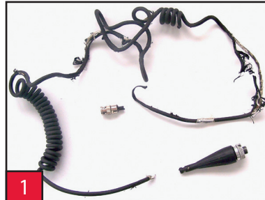
1 In this case, both ends of the cable were destroyed and a serious injury could have happened.
