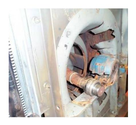
A lack of lubrication was the root cause of this catastrophic bearing failure.
