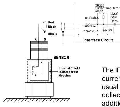
The IFPF constant current power source is usually built into the data collector, and no additional electronics are required.
