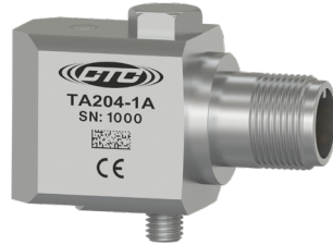
TA204 100 mV/g 10 mV/°C Temp Range: -40 °F to 250 °F -40 °C to 121 °C
