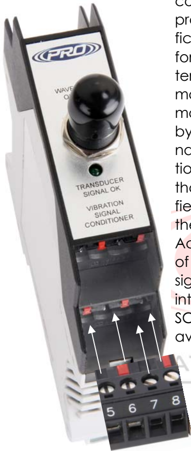
Figure 1; Positions 5-8 Arrows indicate proper alignment of the red keys on receptacle align with open slots on terminal block. Keyed slots on terminal block align with open slots on receptacle.
