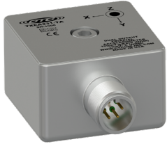
TXEA331-TA Dual Output Triax Acceleration & Temperature 100 mV/g 10 mV/°C
