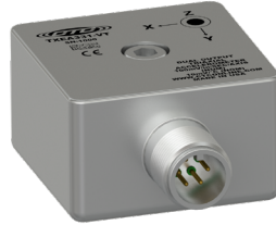
TXEA331-VT Dual Output Triax Velocity & Temperature 100 mV/in/sec 10 mV/°C
