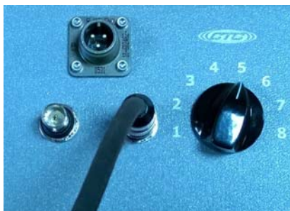
Figure 2— DSB Module showing TM1018 cable connected to test temperature circuit only.
