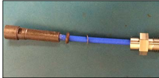
Figure 2— Improved probe tip and case ready for final assembly. Note the o-ring at the back of the molded portion of the probe tip.
