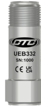
UEB332 Dynamic Vibration IEPE Ultrasound Sensor, 1/4-28 Mounting, Top Exit 2 Pin Mini-MIL Connector, 100 mV/g, ±10%
