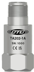
TA202 Dual Output Sensor, Temperature & Acceleration, Top Exit 3 Pin Connector, 100 mV/g, 10 mV/°C, ±10%
