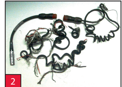
2 In this case, the safety connector saved the data collector and prevented a serious injury!
