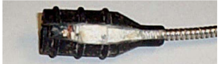
Figure 2; The aluminum back shell inside this boot style connector originally provided a rigid core for the boot to be fitted over. Caustic soda used in the manufacturing process has leaked around the boot and caused the aluminum to corrode and expand, thus weakening the boot, and total failure was the result.
