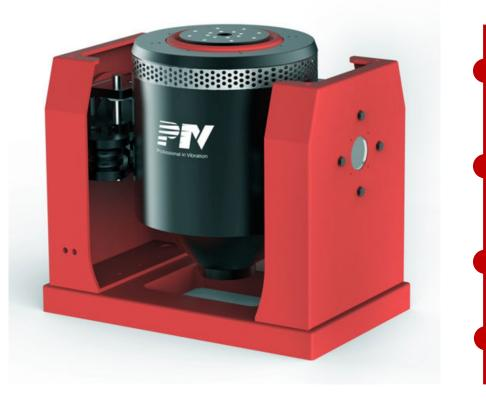
A vibration shaker with a calibrated standard reference accelerometer built into it will be used to simulate the machine vibration.
