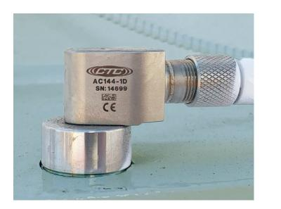
Under ideal circumstances, the accelerometer mounting method should provide total use of the the transmission region.
