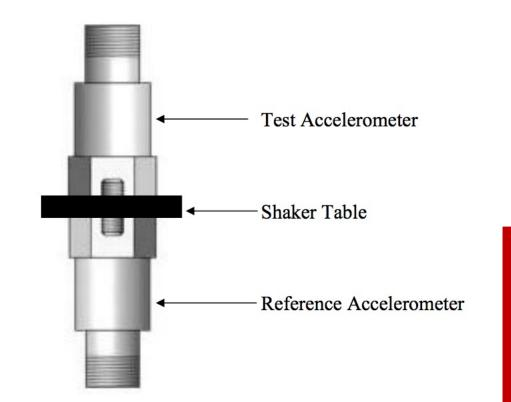
Stud mounting is accomplished with a drilled and tapped hole using a threaded fastener between the accelerometer and the machine.
