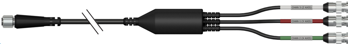
CB105-J4C-020-F3D 4 Conductor, Shielded Cable with Black Polyurethane Jacket, 0.25 in. (6.4 mm) OD, 250 °F (121 °C) Maximum Temperature; Connector 1: 4 Socket Mini-MIL Connector with Rubber Bending Strain Relief, Polyurethane Molded; Connector 2: 3 Channel BNC Plug Connector, Polyurethane Molded
