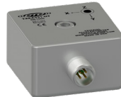
High Temperature Triaxial Accelerometer, Side Exit 4 Pin Mini-MIL Connector, 100 mV/g, ±5%
