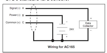
Typical circuit for AC165, note the separate signal and power conductors with a shared common.
