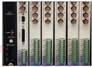
Typical Rack mount input/output cards that can accept AC165 signal/power configurations.
