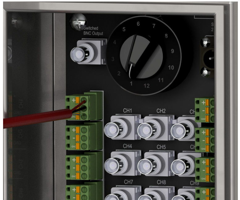
Figure 10. Connecting Cables to Switch Box
