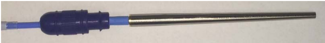
Figure 11 - Sliding connector protector over connector
