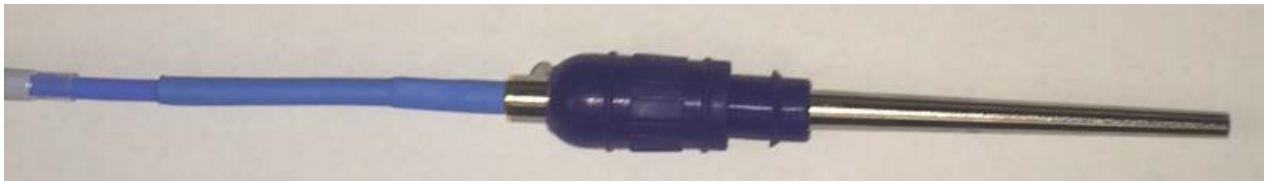
Figure 10 - Sliding connector protector up tool
