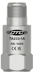
TA233 Dual Output Sensor, Temperature & Acceleration, Top Exit 3 Pin Connector, 500 mV/g, 10 mV/°C, ±10%
