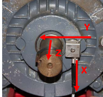
Figure 2—Same sensor, same motor— Different orientation of the X and Y axes.
