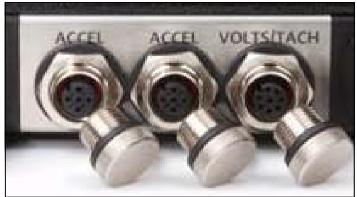
Input ports for CSI 2140 data collector showing 2 separate 5 pin acceleration inputs and one 8 pin voltage/tachometer input port.
