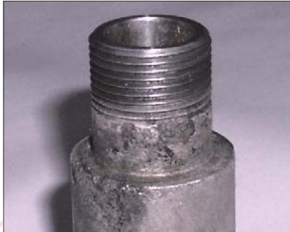
Stainless Steel sensor body showing the effects of corrosion from sulfuric acid.
