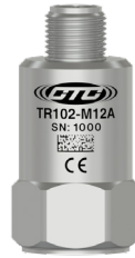
TR102-M12A 100 mV/g PT100 RTD Temp Range: -40 °F to 250 °F (-40 °C to 121 °C)
