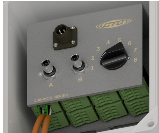
Figure 11. Connecting Cables to Modular Switch Box (DSB3001)
