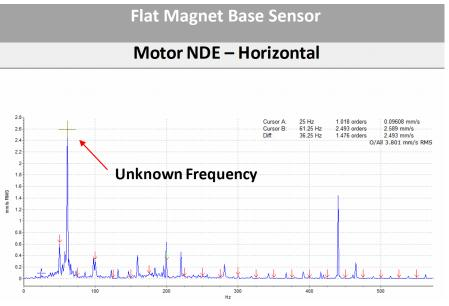
The spectrum is showing higher vibration levels. The spectrum is showing elevated vibration peaks at (61 Hz) which is not seen at any other measurements. The spectrum is showing an attenuation for the vibration data at medium and high frequencies.
