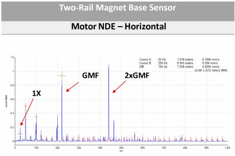
The spectrum is clearly showing vibration peaks at 1x motor running speed and 9x gear mesh frequency with harmonics.
