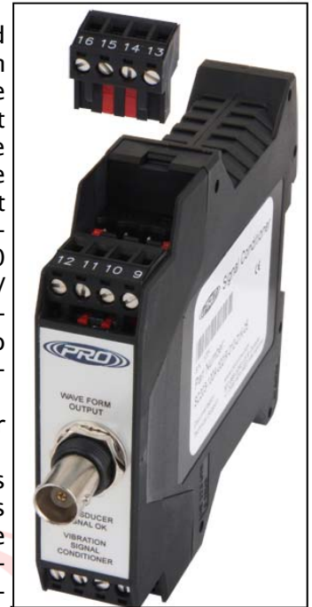
SC200 series Signal Conditioner. Provides 4-20 mA and 0-5 V or 0-10 V outputs proportional to vibration
