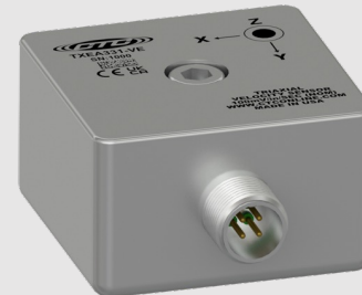
TXEA330-VE Series 100 mV/in/sec, Piezo Velocity, \pm 5\% or \pm 15\% Sensitivity Options
