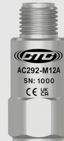
AC292-M12A 100 mV/g, ±5% Sensitivity, Top Exit
