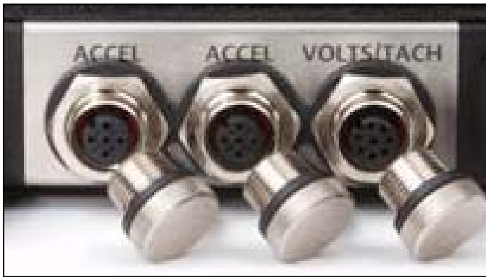
Input ports for CSI 2140 data collector showing 2 separate 5 pin acceleration inputs and one 8 pin voltage/tachometer input port.
