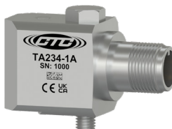
TA234 Dual Output Sensor, Temperature & Acceleration, Side Exit 3 Pin Connector, 500 mV/g, 10 mV/°C, ±10%
