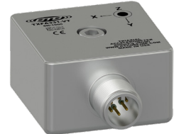
TXFA331-VT Premium, piezo velocity and temperature output, 500 mV/in/sec, 10 mV/°C, ±5%
