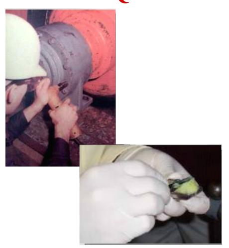
After an analyst decides which mounting hardware is best for the particular application, it is important that the proper technique for mounting the sensor and / or pad is used.
