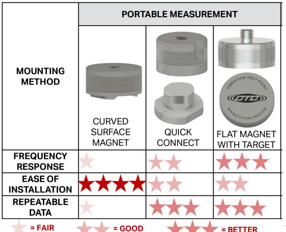
The area of a curved surface (or '2-bar') magnet is not as good as a quick connect system or a flat magnet with a target, and its mass tends to be higher; therefore analysts should not depend on data above the 2 kHz (120,000 CPM). A flat magnet on a well-installed target can yield reliable data up to 8 kHz and possible 10 kHz (600,000 CPM)!
