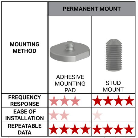
Assuming proper techniques have been used to mill the surface and affix the sensor, permanent mounting options tend to produce good results at higher frequency ranges (up to the full useful range of the sensor). The data will generally be cleaner, more accurate, and highly repeatable.
