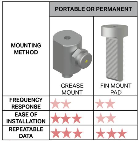
Specialty mounts, such as grease fitting mounts (also known as Zerk adapters), and motor fin mount pads, tend to add a bit of mass, and lack some stiffness. Regardless, they tend to provide good data – usually in the 2 kHz (120,000 CPM) to 5 kHz (300,000 CPM) range – because they are positioned in good proximity to the source of bearing vibration.
