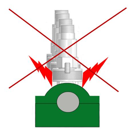
**Don't allow your sensor to be slammed** onto the mounting surface.
