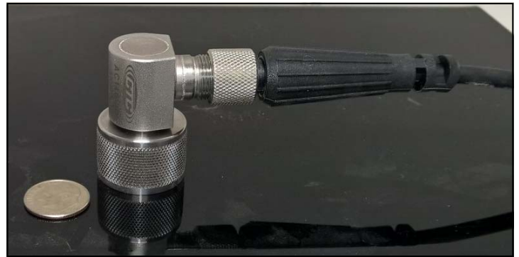
Figure 3—AC146-1D small portable sensor mounted on MH122-1A magnet with J2C cable connection.
