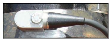
Sensor mounted on pump—Note the paint has been removed and a flat spot has been milled into the surface of the flange for better data transmission.
