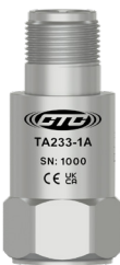
TA233 Dual Output Sensor, Temperature & Acceleration, Top Exit 3 Pin Connector, 500 mV/g, 10 mV/°C, ±10%
