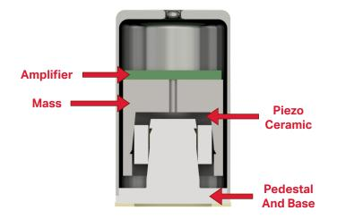
In a shear mode design, no stud holds the internal components together. Most designs use a form of epoxy cured under heat to maintain structure. The base and the mass have no contact, so there is no metal-to-metal contact within the sensing element, which significantly reduces the impacts of thermal transients.
